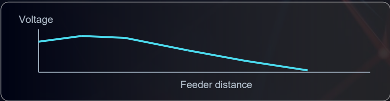
Figure 4: Voltage profile at peak PV output.
